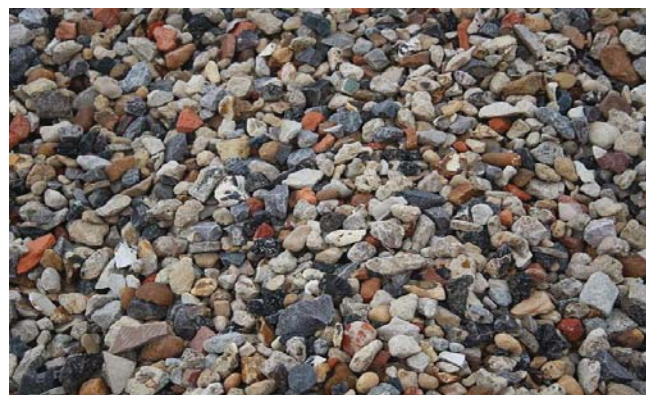
Figura 3.10 Agregate reciclate mixte (10-20 mm)
