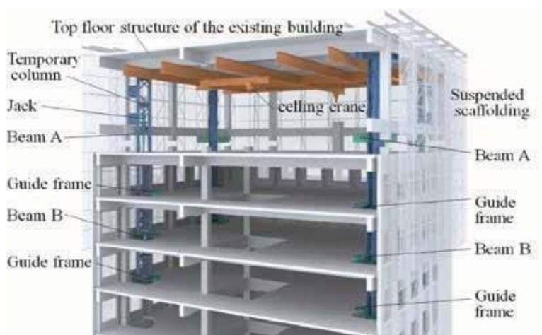
Figura 3.12. Sistemul TECOREP (Sursa: Taisei Corporation)
